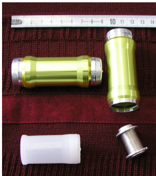
Fig. 10. Rabbit system irradiation capsules, made of thin-walled aluminium for PNA and of polyethylene for NAA.
